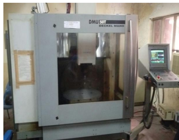
Fig2.3 : Vertical milling machine used for FSW
